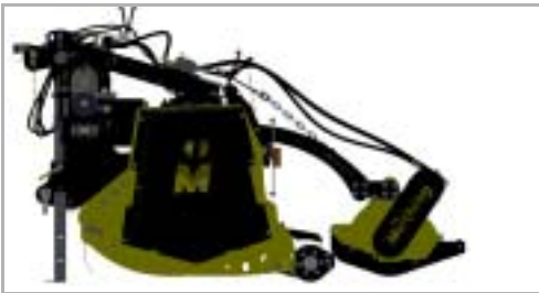
Installation behind the mulcher, with support roller
